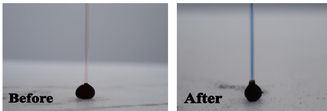
Figure 7. The color change in the DMPD solution inside B-MLMs before and after exposure to \text{H}_2\text{S} gas (60 mg/L).
