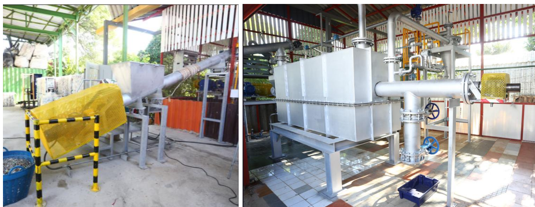
Figure 2. Compound of the single screw pyrolyzer; conveyor (left) and reactor (right)
