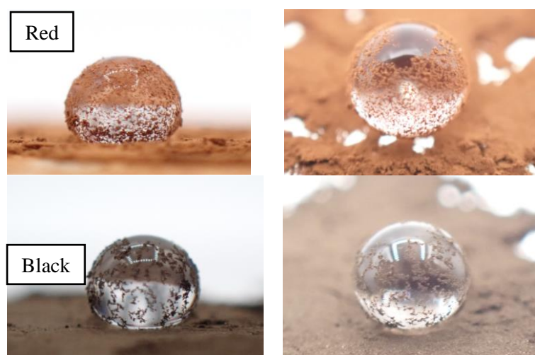
Figure 5. Formation of Magnetic Liquid Marbles (MLMs). The upper row shows red MLMs (R-MLMs), while the lower row shows black MLMs (B-MLMs).
