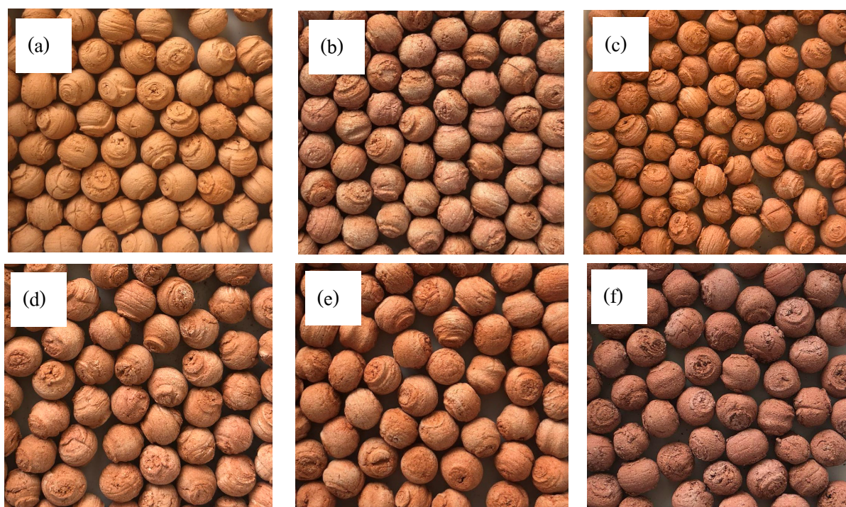
Figure 1. Green and fired ceramsite (a) Pattani clay, ceramsite containing 70 % Pattani clay, 20 % fly ash and 10% (b) cockle shell; (c) tapioca starch; (d) rice husks; (e) sawdust; and (f) iron(III) oxide, after calcined at 1,000°C.
