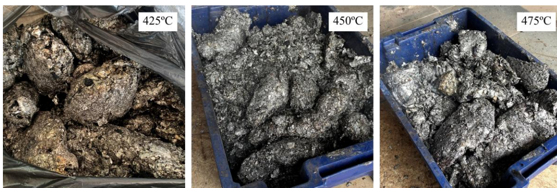
Figure 3. Physical property of solid product after pyrolysis process through single screw reactor in each operating temperature; 425, 450 and 475°C, respectively
